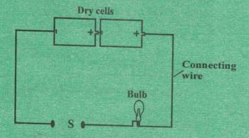
Material E when used to connect wires at position S would make the bulb not light and material F would make the bulb light.
