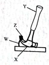
Which one of the following parts labelled W, X, Y, Z shows the position of fulcrum while the lever is in use?
