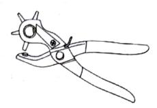
The tool in the picture above is used in; A. weaving B. cutting C. carving D. leather work.
