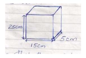
Given that the weight of the block is 25N.Determine:(i) The maximum pressure it exerts on the surface(3mks)
